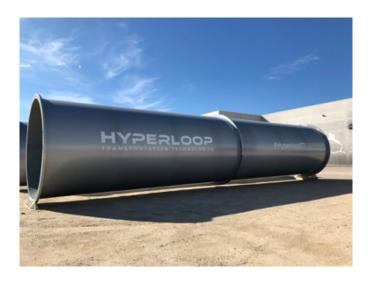
painted with a coat of Hempel Galvosil 15700, an inorganic zinc silicate made up of two components which offers outstanding resistance against damage of all varieties.
